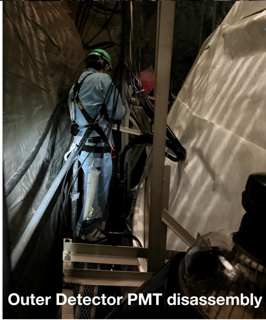
Outer Detector PMT disassembly
