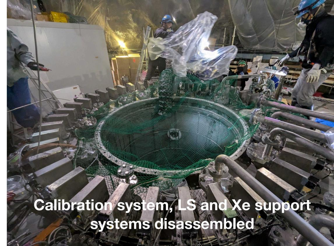
Calibration system, LS and Xe support systems disassembled
